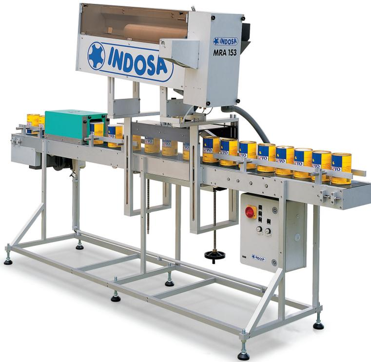
**Automatic line for applying of snap-on lids to cans**
